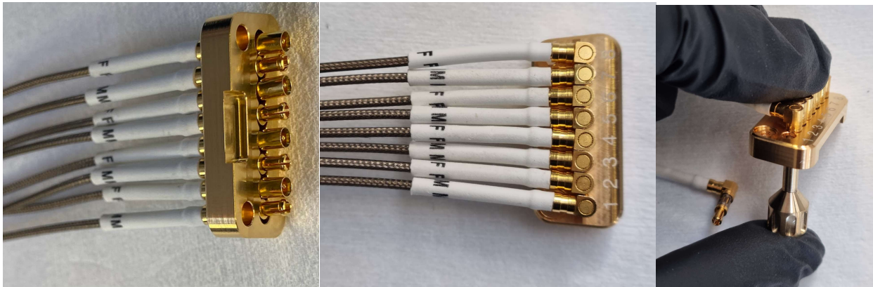
Figure 7 Left) Eight straight coaxial cables clicked into a face-plate. Middle) Eight Right-angled coaxial cables clicked into a face-plate. Right) Extraction tool (Q425) used to remove the individual connections from the face-plates.
