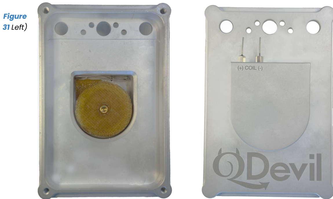
Superconducting magnet coil mounted. Right) DC current supplied via filtered feed-throughs inside the superconducting shield
