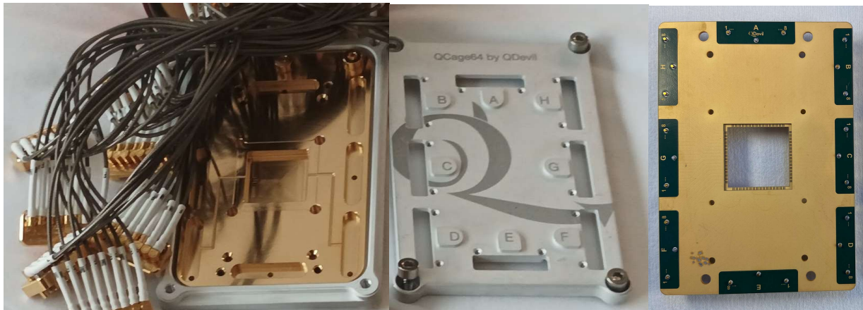
Figure 19 Left) The EMC tight cavity. Middle) The aluminum top cover. Right) The sample board.
