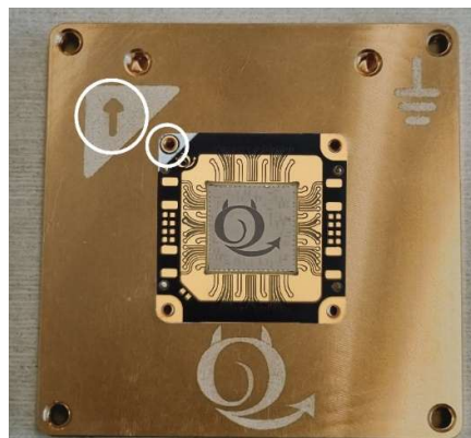
Figure 21 – The sample board is aligned by a white triangle to the grounding plate (QBRD2-GND)
