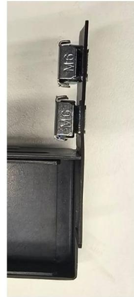
4. **Position right rail assembly:** Place the right rail assembly (MP0286) in the appropriate location in the rack. The rail assembly should be attached to the inner side of the rack beams.
