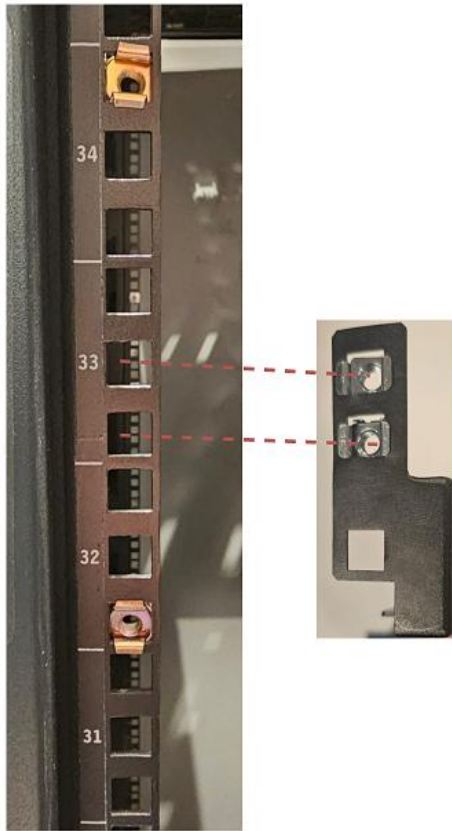
Picture 4 – Front side view of the rack with the rail assembly location indicated
