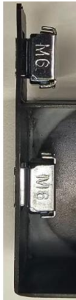
Picture 2 - Back side of the rail assembly with cage nuts installed
