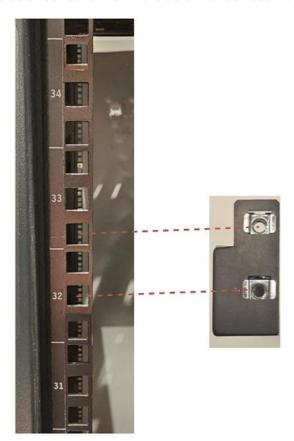
Picture 5 – Back side view of the rack with the rail assembly location indicated
