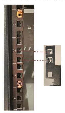
Picture 4 – Front side view of the rack with the rail assembly location indicated
