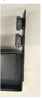
Picture 2 - Back side of the rail assembly with cage nuts installed
