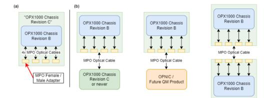
Figure 4 - (a) Connecting the four MPO Optical cables and 4 MPO adapters converts a Revision B chassis into a Revision C chassis. (b) Using the adapters allows connecting the chassis to other products
